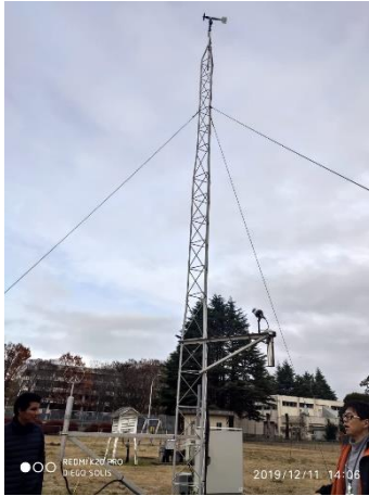
Figure 79. Automatic meter station.
